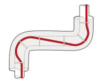
• Support: For uninsulated pipe supports, allow twice the length of the support, plus an additional 16" (40 cm) of heating cable. Install the heating cable in a loop, following as a guide. Insulated pipe supports do not require additional length of heating cable.
